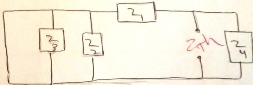
$$Z_{th} = \frac{7.211 \angle -56.309^\circ \times 2}{6 - j6} = \frac{14.422 \angle -56.309^\circ}{8.485 \angle -45^\circ}$$
